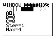
After designating the settings, press GRAPH . The TI-84 computes the screens that show the function changing dynamically. To pause the graph, press ENTER . To reactivate it, press ENTER again. To stop the graph, press ON, which returns the you to the SETTINGS Screen.
